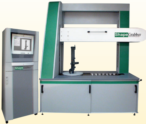
The ShapeGrabber Ai810 scanning an automotive radiator component
