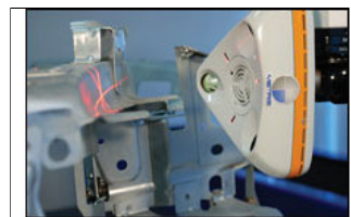
Metris offers several variants of laser-line scanners, such as the new XC65D with advanced processing capabilities, for integration with CMMs.
