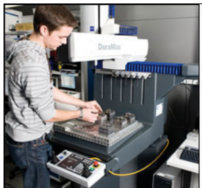
The DuraMax from Carl Zeiss IMT is a turnkey CMM used to replace hand-gaging for flexibility, speed, and accuracy.
