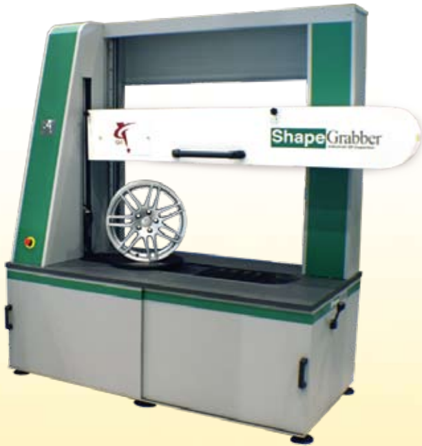
The ShapeGrabber Ai810 scanning system
